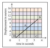
For example, velocity at A is  $\frac{\overline{BC}}{DC} = \frac{(8-2)m}{(3-1)s} = \frac{6}{2} \frac{m}{s} = 3m/s$ .
